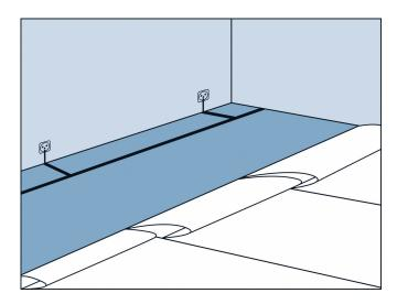
**Attention:** Only use coverings with horizontal conducting back coatings. The copper tape may show through the floor covering.
